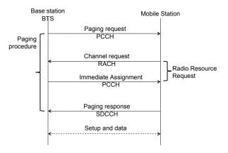
Figure 2. Sequence diagram for the first 4 messages in the paging procedure over the air interface between the BTS and the MS.
