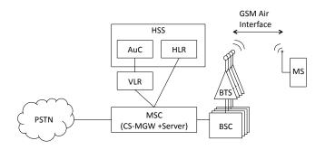
Figure 1. Simplified diagram of a cellular network connected to the PSTN. Only nodes relevant to this work are shown.
