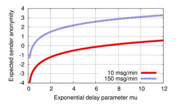
Figure 11. Expected sender anonymity for varying delay parameters with the lowest observed traffic rate of 10 messages/minute and the highest observed traffic rate of 150 messages/minute.
