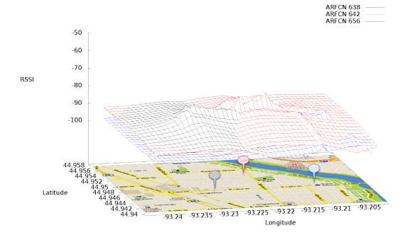
Figure 10. Signal strengths for 3 ARFCNs in a 1.5  $\times$  2.5km area. The peaks of the meshes correspond directly to the geographic position of the observed BTS.
